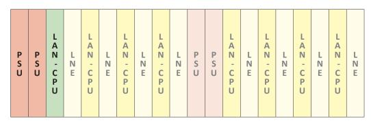
**Sample 1:** max. 8 x LAN-CPU with 8 x LNE, max. 40 network interfaces
