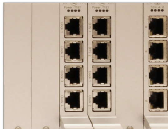
Figure: LIU modules in 3HE IMS chassis with balanced Clock and BITS outputs (RJ45 connectors)
