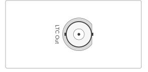
Cable: Coaxial Cable, Shielded
