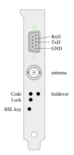
The bracket of the board includes the BNCconnector for the amplitude modulated time codes, three LEDs, a key for activating the Bootstrap- Loader and a 9 pin D-Sub-plug.
