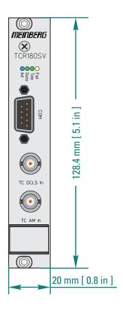
The frontpanel of the board includes the BNC connector for the amplitude modulated time codes, four LEDs and a 9 pin D-Sub-pluq.
