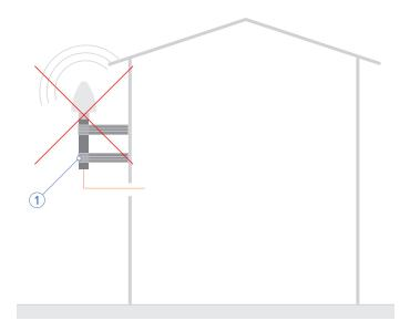
Fig. 2: Poor positioning of a wall-mounted antenna (1)
