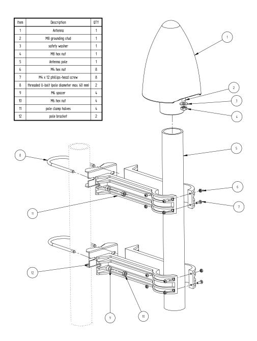
Fig. 3: Mounting a Meinberg GPS Antenna onto a Pole
