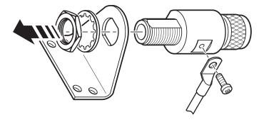
Fig. 7: Installation of the Surge Protector
