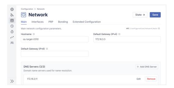
As soon as the Dashboard appears, open the "Configuration" section in the header bar and select the subsection "Network". You should ensure in particular that the network configuration is performed for the intended management interface ("Interfaces" tab) to ensure that it is accessible from the subnet.
