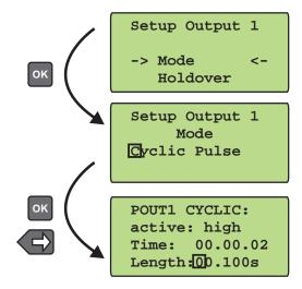
The value in field **Time** determines the time between two consecutive pulses (2 sec in example above). This cycle time must be entered as hours, minutes and seconds. The pulse train is synchronized at 0:00 o'clock local time, so the first pulse of a day always occurs at midnight. A cycle time of 2 seconds for example, would cause pulses at 0:00:00, 0:00:02, 0:00:04 etc.
