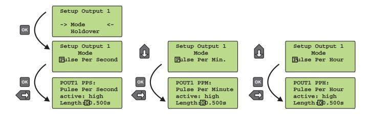
These modes generate pulses of defined length once per second, once per minute or one per hour. **Time** determines the pulse duration (10 msec...10 sec).
