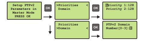
In "Unicast Master" mode, only the priority1 and priority2 values and the domain number can be configured. Furthermore, the "Unicast Negotiation" feature is supported when operating as grandmaster, therefore all Unicast specific message parameters have to be configured on the Slave.
