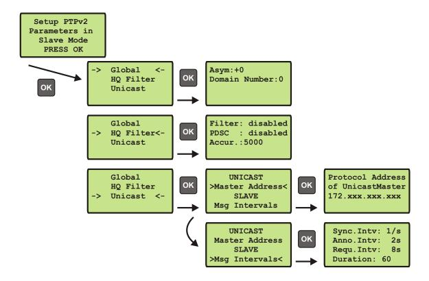
In addition to the parameters that have been already described in chapter "PTP Parameters", the following values can be changed in Unicast Slave mode.
