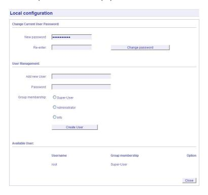
The menu "User Management" allows you to set up different users with a password and the group membership. To change the properties of an user you have to delete the old user and set up a new one. The user "root" cannot be deleted and has always the membership of Super-User. The password of the user "root" can be set on the security page.
