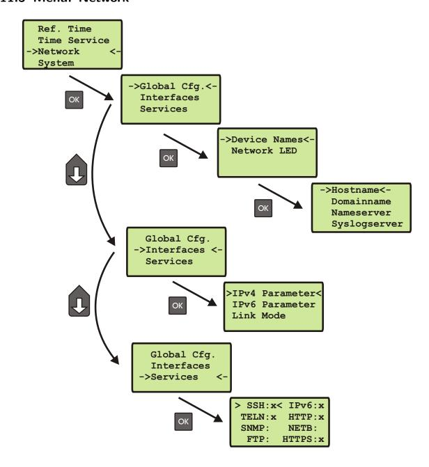
In this submenu the network configuration parameters related to the network interfaces can be changed. The submenus can be selected with the arrow keys and the "OK" button:
