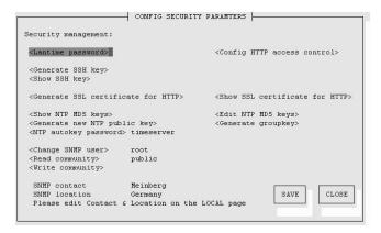
The password is stored encrypted on the internal flash disk and can only be reset to the default value "timeserver" by a "factory reset", changing all settings back to the factory defaults. Please refer to the LCD configuration section in this manual.
