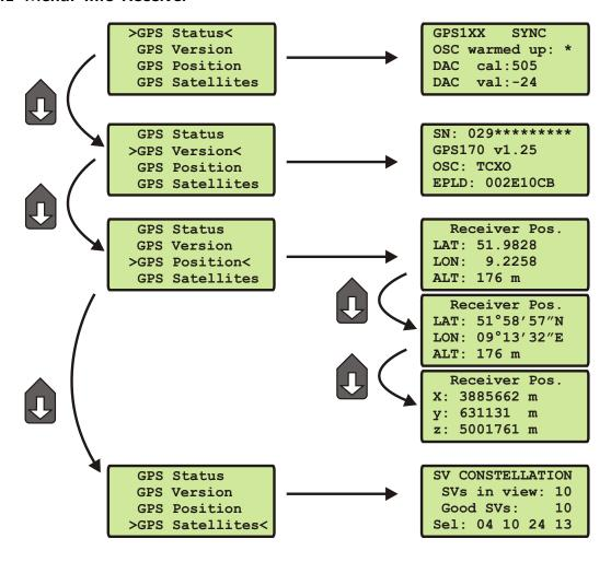
In this menu all relevant information about the GPS radio clock, the internal oscillator and the GPS satellites will be shown.
