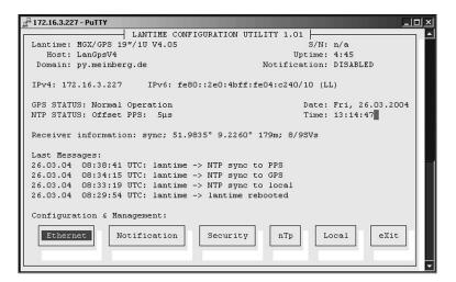
In addition to the SNMP and web interface, you can also manage your LANTIME configuration via a command line interface (CLI), which can be used via a TELNET or SSH connection. A setup tool can be started after login, just type "setup" and press ENTER at the prompt.
