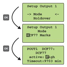
In 'DCF77 marks' mode the selected output simulates the telegram as transmitted by german time code transmitter DCF77 (see chapter DCF77 Emulation in radioclock manual). The generated time code is related to the local time zone.
