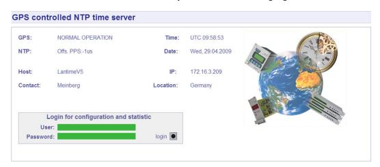
On this start page you see a short status display, which corresponds with the LC display on the front panel of the LANTIME unit. The upper line shows the operation mode of the receiver.
