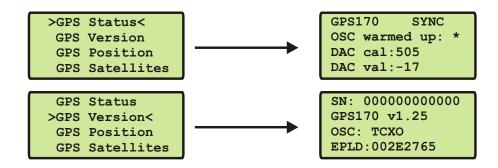
The second line of "GPS Version" will reflect the version number of the GPS reference clock and the oscillator type. In the bottom line the serial number of the receiver will be shown.
