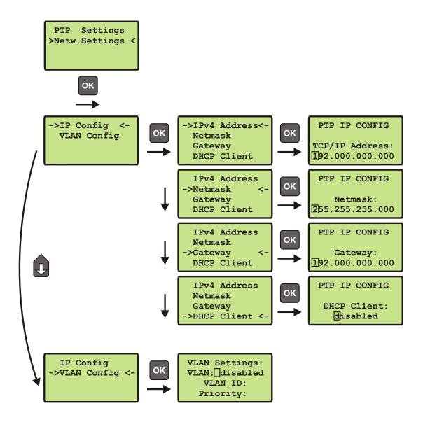
IP configuration for the PTPx interface. It can be selected if either a static IP address shall be used or if a dynamic IP address via DHCP should be assigned.
