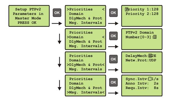
In addition to the already described parameters which can be found above in the chapter PTP Parameters, the packet rate of the Sync, Announce and Delay Request messages can be configured here (64/sec...64 sec).
