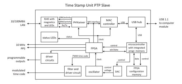
After decoding valid time information from a PTP Master, the system sets its own PTP seconds and nanoseconds accordingly. The PTP offset calculated by the PTP driver software of the single board computer is used to adjust the master oscillator of the TSU-USB. This allows the PTP Slave to generate very high accuracy output signals (10 MHz/1PPS/IRIG).
