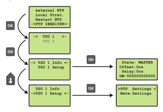
The menu for PTP IEEE 1588 configuration is located under the "Time Service" main menu and is divided into "TSU x Info" and "TSU x Setup". A device with more than one PTPv2 card (also called as "TSU", Time Stamp Unit) lists all cards in this sub menu.
