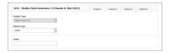
In the menu "IO Configuration" you can set the output on DARS for every output of the IMS LANTIME M3000S. The four available outputs can optionally be switched off.
