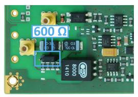
Figure 1: Jumper Settings: 600  $\Omega$
