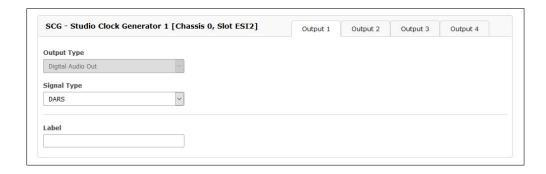
In the menu "IO Configuration" you can set the output on DARS for every output of the IMS LANTIME M2000S. The four available outputs can optionally be switched off.
