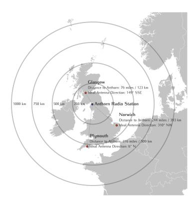
Illustration: Installation of how an AW02-60 antenna is directed towards the MSF transmitter tower in Anthorn, Cumbria, UK from various locations in the UK.
