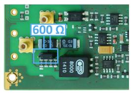
Figure 1: Jumper Settings: 600  $\Omega$
