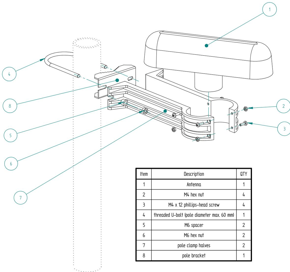
*Illustration: Mounting an AW02 antenna onto a pole*
