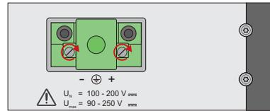
Illustration: Lock screws on an MSTB plug connector; in this case on a LANTIME M320
