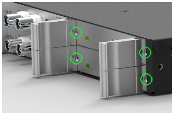
Figure 7.9: Locations of fixture screws in a 1U IMS LANTIME system
