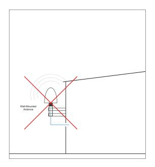
Fig. 2: Poor positioning of a wall-mounted antenna
