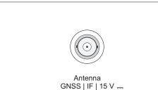
This intermediate frequency is the result of the downconversion from the original L-band GNSS frequency by the GPSANTv2.
