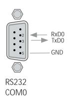
The serial port COM0 is accessible via a 9pin DSUB male connector in the frontpanel of the GPS180, parallel hardwired to the COM0 port on the rear VG edge connector.
