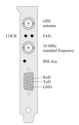
The coaxial antenna connector, two status LEDs and a 9 pin sub D connector can be found in the rear slot cover. (see figure). The upper, green LED (LOCK) is turned on when after power-up the receiver has acquired at least four satellites and has computed its position. In normal operation the receiver position is updated continuously as long
