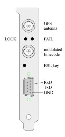
The coaxial antenna connector, two status LEDs and a 9 pin sub D connector can be found in the rear slot cover. (see figure). The upper, green LED (LOCK) is turned on when after power-up the receiver has acquired at least four satellites and has computed its position. In normal operation the receiver position is updated continuously as long
