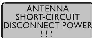
If this message appears the clock has to be disconnected from the mains and the defect is to eliminate. After that the clock can be powered-up again. The antenna supply voltage must be in a range of  $18.5V_{DC}$  (free) and  $16V_{DC}$  (connected GPS antenna).
