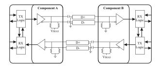
This design leads to a full duplex connection clocked with 2.5 GHz capable of transfering a data volume of 250 MB/s per lane in each direction. Higher bandwith is implemented by using multiple lanes silmutaneously. A PCI Express x16 slot for example uses sixteen lanes providing a data volume of 4 GB/s. For comparison: when using conventional PCI the maximum data transfer rate is 133 MB/s, PCI-X allows 1 GB/s but only in one direction respectively.
