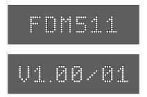
Knowledge of the firmware revision is helpful whenever technical support from Meinberg is needed. The **Menu** button is used to skip to the menus described in the following. The corresponding content of the menu is displayed after selection is done with the **Set** button.
