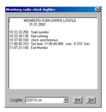
Submenu **View logfile** opens a window showing the current logfile. All other files may be displayed by selecting them from the list at the bottom of the window. Using the "Ref" button causes an update of the present-day logfile, using the "Del" button deletes the displayed file.
