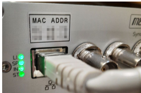
Illustration: MAC address printed above the network port
